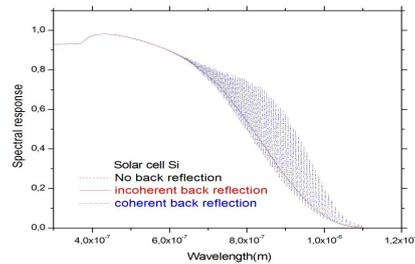
Fig. 2 show the curve of the spectral response for the solar cell based of Si.
